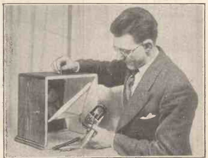
The final operation in the construction of the cabinet cone is mounting the batten for supporting the unit. This consists of a strip of wood, which is screwed into position, as shown above.
