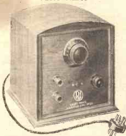
The adaptor is built into a very neat cabinet, and it is connected up to the broadcast receiver by means of the special plug provided.
