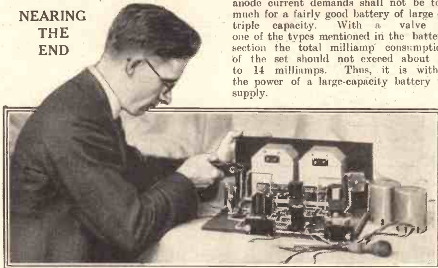
Like a wise constructor he is going round with a pair of pliers to make sure that all the connections are properly tightened.
