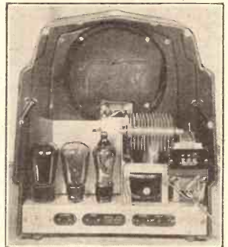
The works of the "EKCO" M.23 A.C. receiver. It is a three-valver and uses a metal rectifier.
