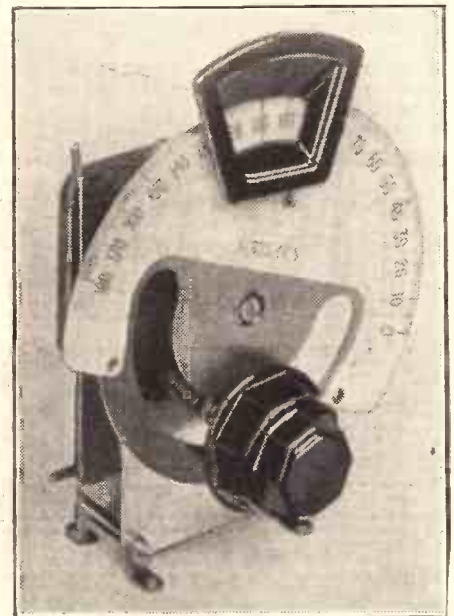
Although at first sight this device looks like a good slow-motion dial, it is actually this plus a two-gang condenser
