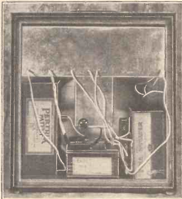
Our new "P.W." Portable is a complete breakaway from the old-fashioned open layout type of design, where merely an ordinary baseboard and panel construction is slipped into a portable cabinet.
