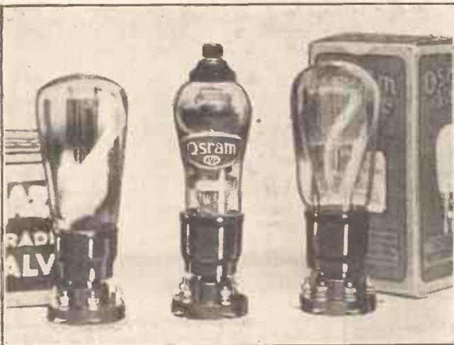
Here are three of the latest D.C. indirectly-heated mains valves. From left to right they are the Marconi D.H., an excellent detector; the Osram D.S., the D.C. version of the M.S.4; and the Mazda D.C./H.L., which is the direct-current counterpart of the famous A.C./H.L.
