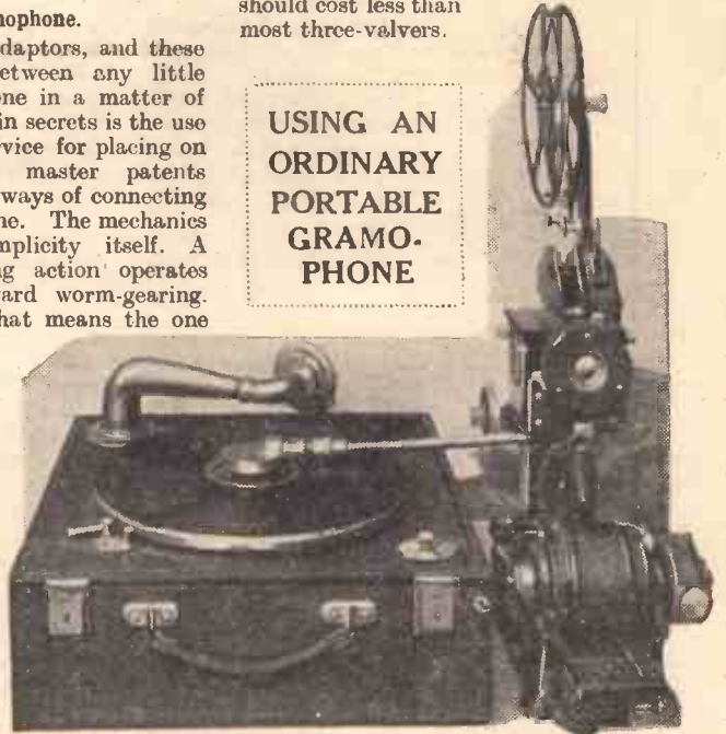
This photo shows a portable gramophone synchronised with a small, inexpensive home cinema machine. Note the simplicity of the scheme. The record can be changed as quickly as in the ordinary way.
