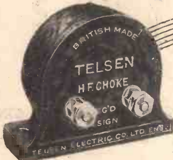
TELSEN H.F. CHOKES. Designed to cover the whole wave-band range from 15 to 4,000 metres, extremely low self-capacity, shrouded in genuine Bakelite. Inductance 150,000 microhenries. Resistance 400 ohms. Price 2/6 each.
