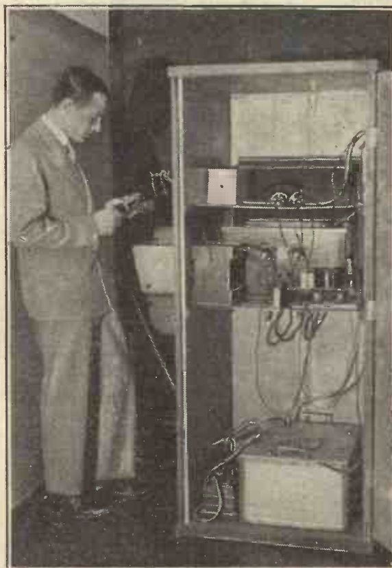
The aperiodic high-frequency power amplifier used by von Ardenne in experiments with his interesting radio programme rediffusion scheme.
