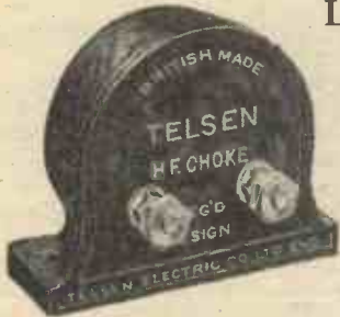
TELSEN H.F. CHOKE. Designed to cover the whole wave-band range, from 18 to 4,000 metres. Extremely low self-capacity, shrouded in Genuine Bakelite. Inductance 150,000 microhenries, resistance 400 ohms. Price 2/6 each.
