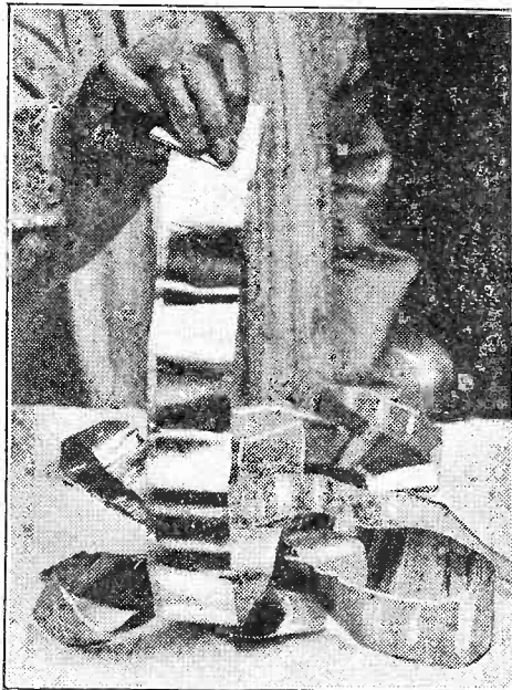
A small section of the gigantic strip of metallised paper used in Mansbridge condensers. There are many yards in a 2-mfd. condenser of this type.
