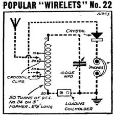
The connections for a good crystal circuit (based on a home-made coil and the other "components" shown last week) are indicated by the dotted lines abov
