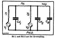
current via C to earth, and should not pass any current to earth via  $V_2$ . If we see  $V_1$  and  $V_2$  with de-coupling resistances (Fig. 2), we see that there is a by-pass to earth of a condenser Cd<sub>1</sub>, and a resistance Rd<sub>1</sub>, each making it more difficult for  $V_1$ to pass a current through  $V_2$  to earth.
