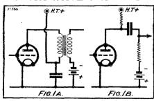
Whereas plain transformer coupling is likely to provide threshold howl, resistance coupling is almost immune from that fault.
