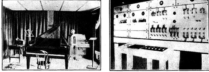
The studio at K U O M and the main switchboard. Between these two the energy representing the speech and music is amplified millions of times by valve magnifiers.
