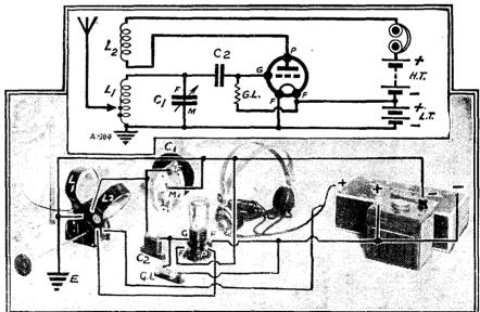
Here is a complete one-valve circuit with "swinging-coil" reaction. The components in the photo are connected up exactly in accordance with the theoretical circuit above, and all the lettering appears in its correct order. See if you can identify all the components and follow out their connections.
