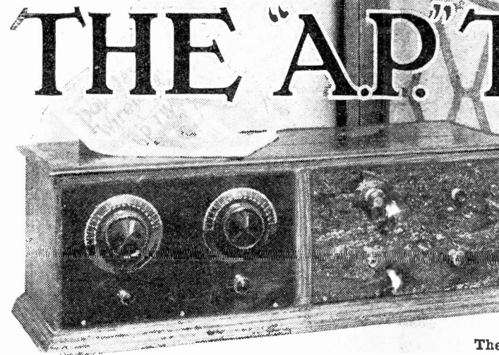
Here is a companion unit to the "A.P." Amplifier; described in "A.P." Two is a really efficient screened-grid and detector receiver stations with remarkable strength. Add it to the amplifier (if desired), and you have a powerful four-valver of first-class quality.
