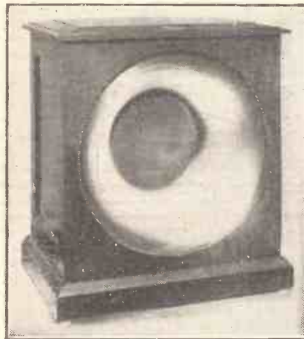
A moving-coil speaker of unusual design is the "Brown."
