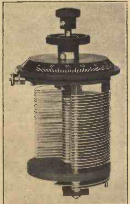
An old-type variable condenser. Note its ebonite end plates and semi-circular vanes.
