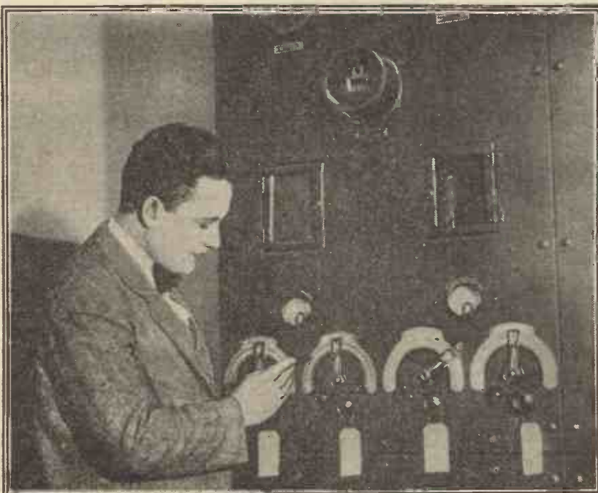
The Engineer-in-Charge of W.E.A.F. (New York) resetting the dials on the amplifier to conform to the new 860-kilocycle wave of that station, which, among many others, was altered by order of the Federal Radio Commission.
