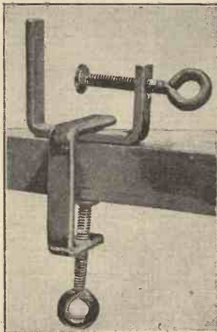
Showing how two clamps of a most inexpensive nature, can be arranged so as to form a useful vice.
