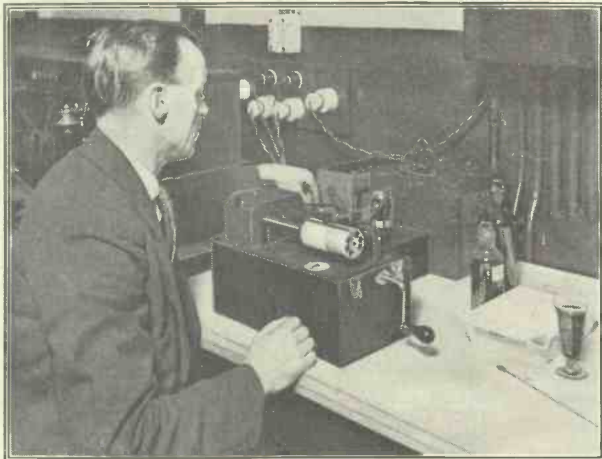
This is the receiving apparatus installed at Savoy Hill to check the pictures broadcast by Daventry (5XX) 76 miles distant.
