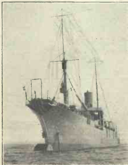
This vessel is the Citta di Milano, that played an important part in the rescue of General Nobile, of the airship "Italia," which was wrecked on drifting ice near the North Pole. Note the elaborate aerial equipment.
