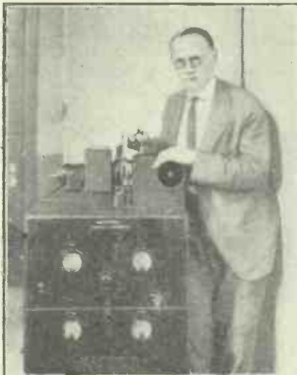
DR. VLADIMIR K. ZWORYKIN, the inventor of the new Radio-photo transmitter. He is shown inserting one of his photo-electric cells into the transmitting apparatus.
