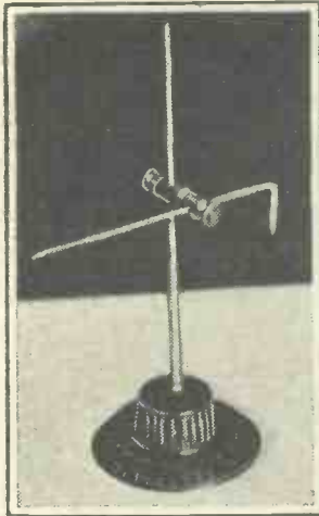
Fig. 1.—The scribing block, which can be made with an old ebonite dial and various small pieces of material that you may have on hand.
