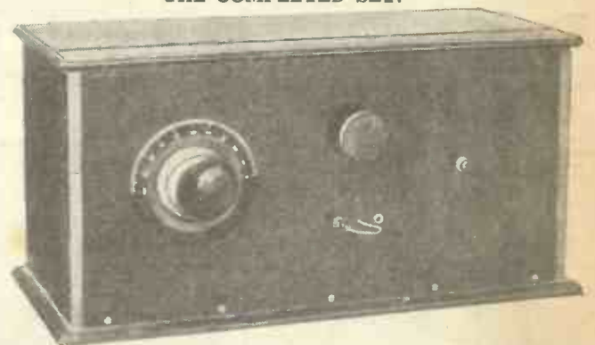
Easy to build and easy to handle, the "Q. and A." Three has only two operating controls—the tuning condenser and reaction adjustment.
