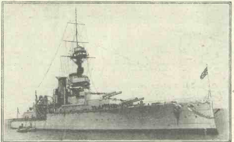
Without a single man on board her, this great warship—H.M.S. "Centurion"—can be completely controlled by radio. She has been equipped by the Admiralty as a target-ship, and by means of the marvellous machinery in her hull she is worked by wireless from another ship, which may be miles away.
