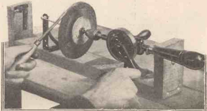
The device in use as a grindstone. The blade of a screwdriver is being sharpened.
