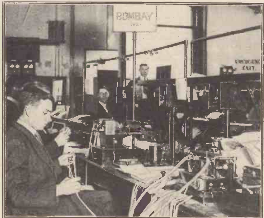
Receiving messages on the automatic telegraph instruments at the London Central office, which arrive via the recently inaugurated Indian Beam service.
