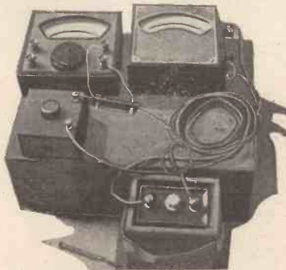
Testing a soldered joint. The joints under test are connected across the two terminals on the ebonite strip. On the left is the millivoltmeter, and on the right is the ammeter. The small square box (left front) is merely a rheostat.
