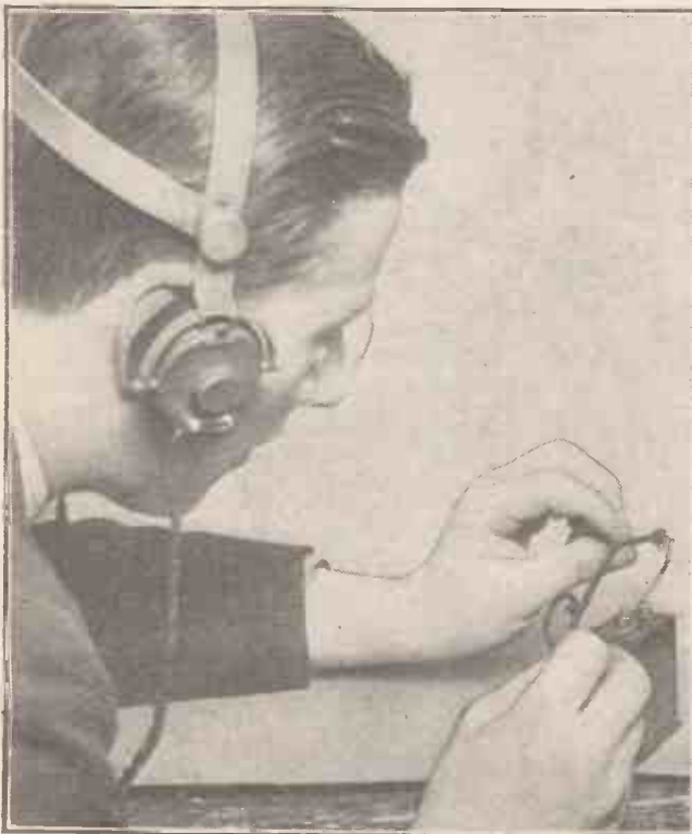
Make sure that fixed condensers are all O.K. and that they do not leak.
