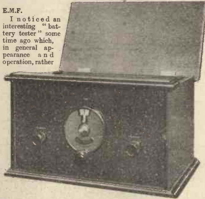
A neat three-valve set, having “ganged” tuning controls, built by one of our London readers.
