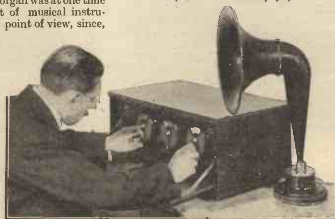
Bringing the set up near the oscillation point, or using too much selectivity, is one way of receiving a programme.
