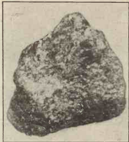
Fig. 3. A natural lump of galena before it is broken up for radio purposes.
