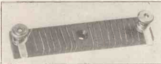
Fig. 1—A ten-ohm resistance element. Photograph is reproducal full size.
