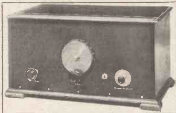
An extremely neat panel appearance characterises the Savoy Three, while the Verno-dial enables very easy tuning to be obtained.
