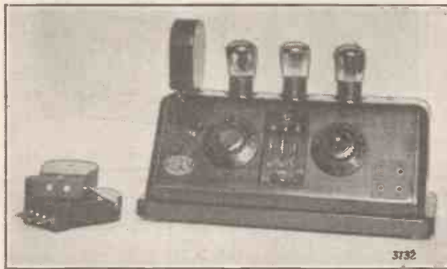
An example of modern receiver design—a popular three-valve set of German manufacture.
