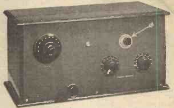
This two-valve Filadyne, described in "P.W." 218, can easily be modified, and there is ample space for the potentiometer on the panel as indicated by the arrow.
