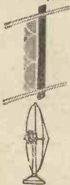
A cone diaphragm loud speaker can easily be constructed. The illustration shows one method of mounting.
