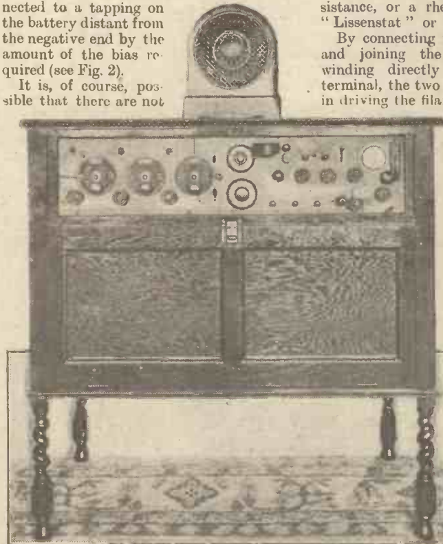
A magnificent set built by an Australian reader, Mr. S. Golding, now in England. Seven valves are employed, 2 neutralised H.F., 1 Det., 2 L.F., and two further stages of push-pull amplification. The lower part of the cabinet contains batteries, wave-meter, and charging system for batteries.
