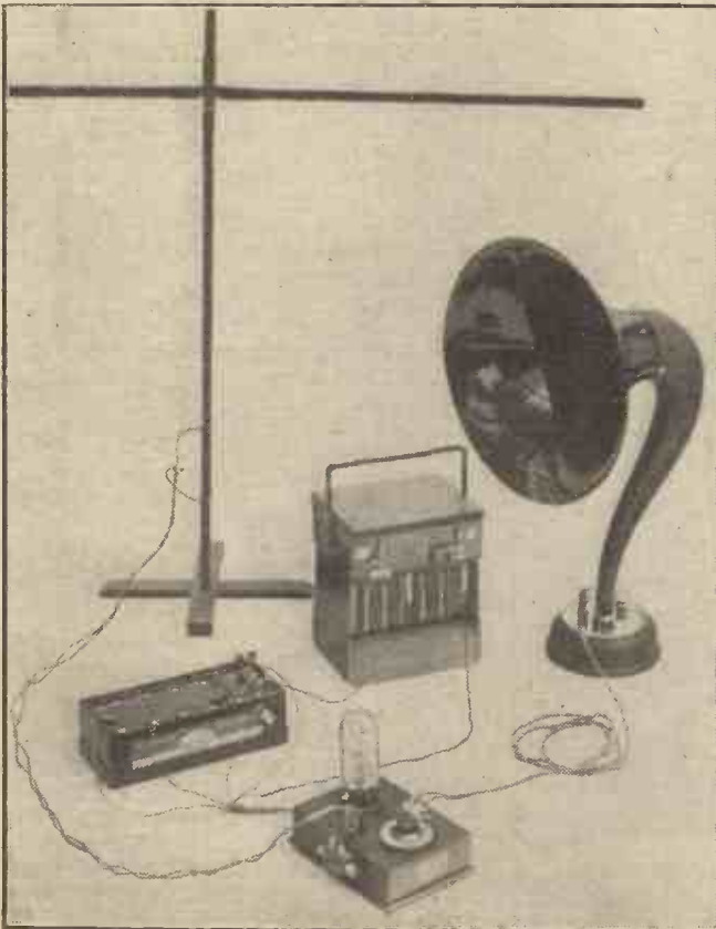
A complete three-valve set, using the new Loewe triple valve.
