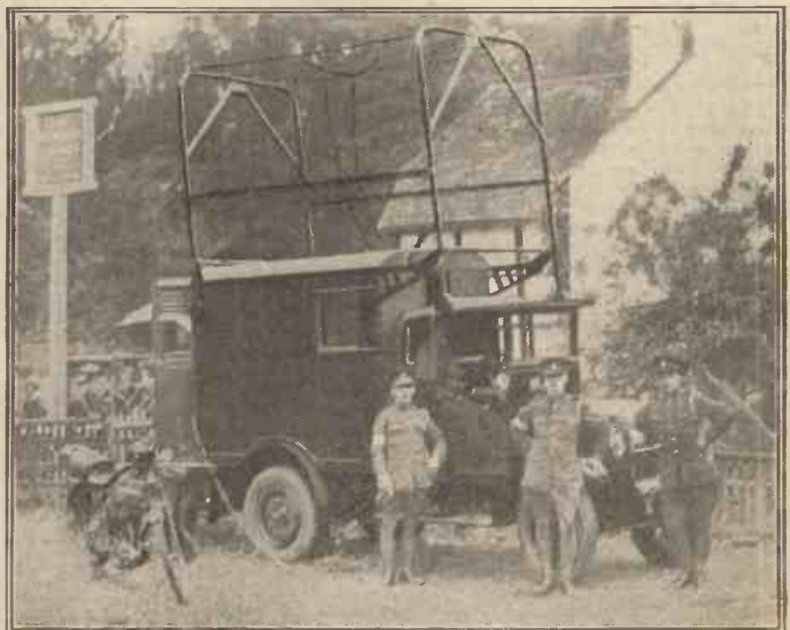
One of the latest army mobile wireless stations together with two of the operators and a driver.
