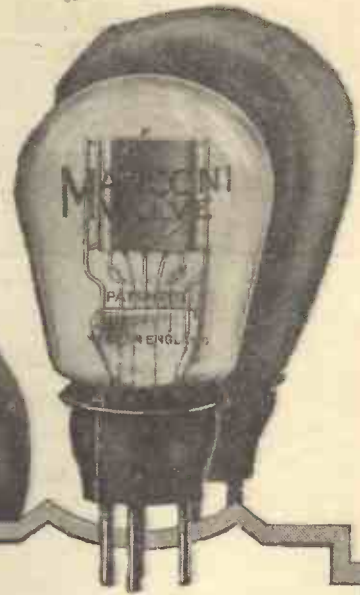
Type D.E.5. A dull emitter for L.F. amplification. Recommended as last valve of amplifier, using R.5V or other valves running from a 6-volt accumulator. Price .. .. 22/6
