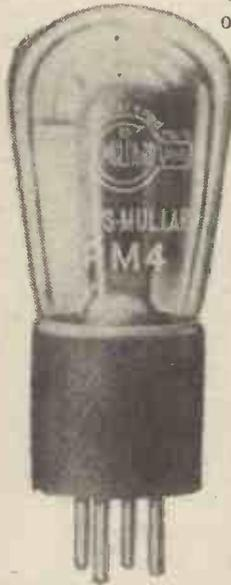
The P.M. 4 Dull Emitter for L.F. Amplification. (Messrs. Mullard.)
