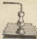
Screw the Soldercup firmly to the Terminal Base. Apply a little Flux to the wire, and hold in position with a little pressure on the solder.
