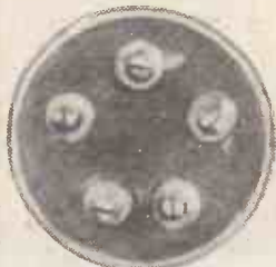
Showing the arrangement of the five pins in the base of the U.C.5 valve.
