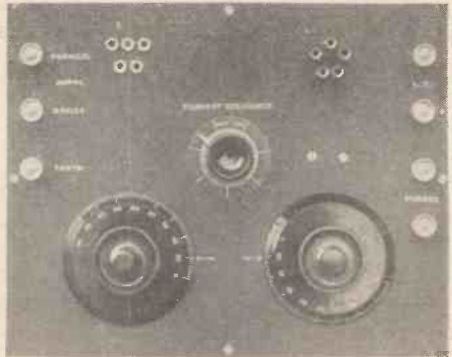
A close-up of the panel face, showing the lay-out of components. The two counter sunk screws beneath the valve sockets hold the choke in place.
