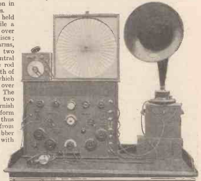
An interesting 4-valve set and home-made loud speaker constructed by Mr. R. S. Rudland, of 36, Gipsy Road, Welling.
