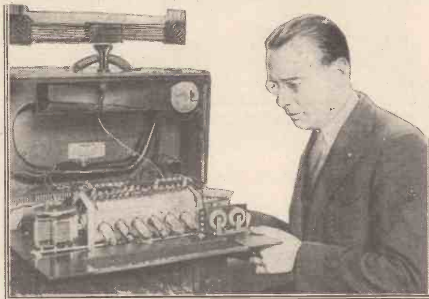
This portable super-heterodyne receiver of American design includes a self-contained loud speaker.
