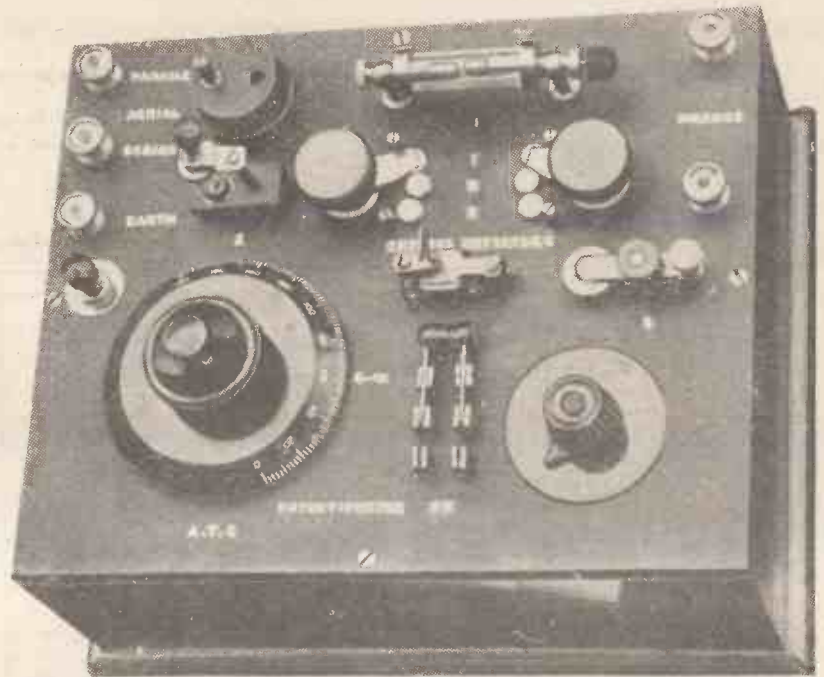
The completed set as will be seen above, is a very compact, neat little instrument. The switches are "set" for the perikon detector, the potentiometer battery being switched off.
