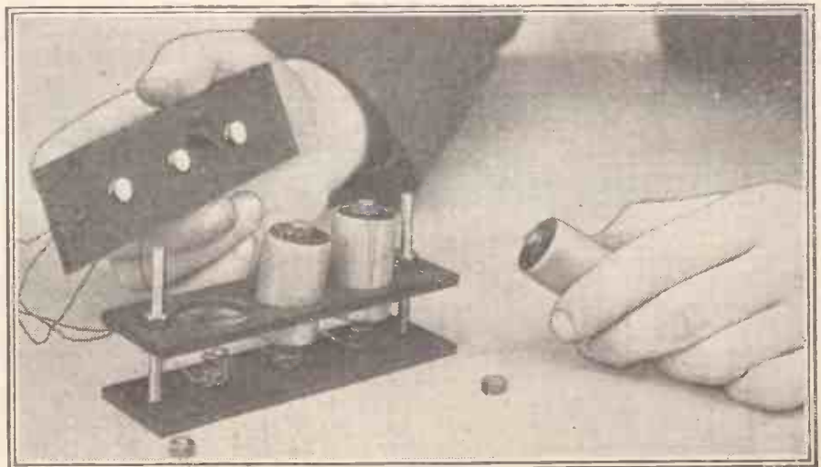
The cells can be quickly removed and changed if the case described is employed.
