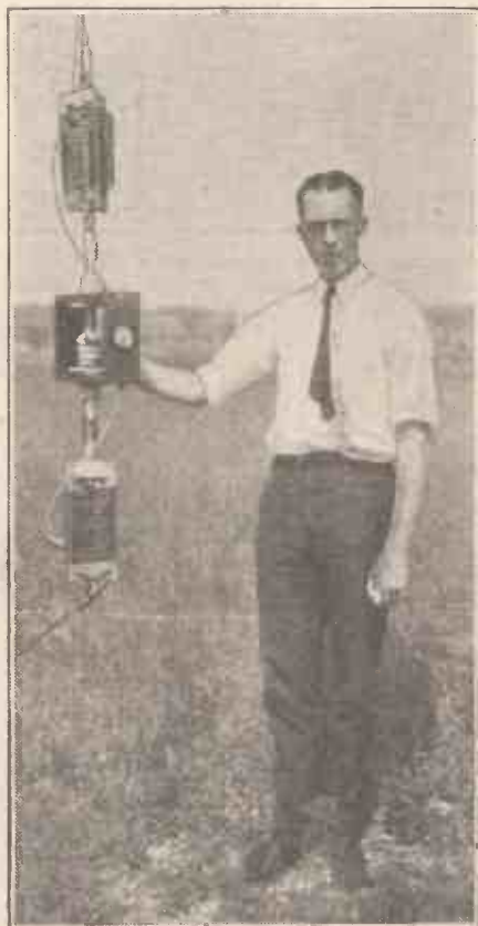
This photograph shows the meter placed in the centre of the 40-metre aerial.
