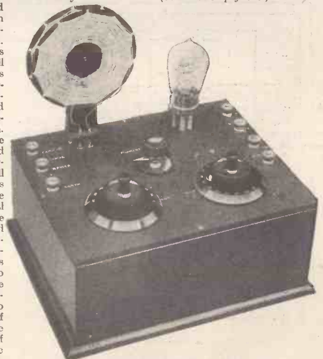
The completed one-valve 1926 Unidyne showing the original type of tuning unit employed.
