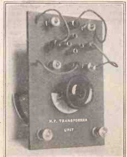
Fig. 20. A useful unit for testing H.F. transformers.
