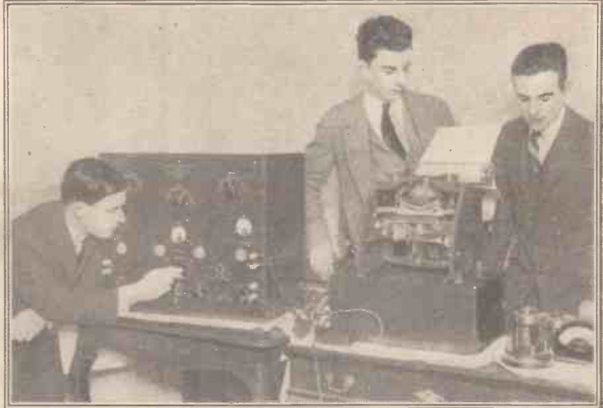
High speed automatic reception of morse code radio signals. This apparatus has been fitted up in the offices of a well-known New York newspaper.
