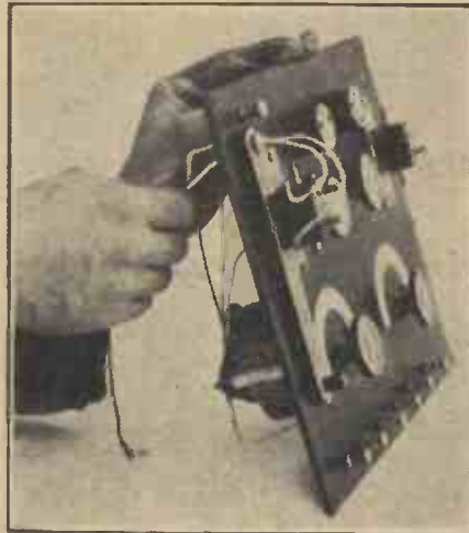
Fig. 16. Connecting up the reaction coil. with 4 volts low-tension current.
