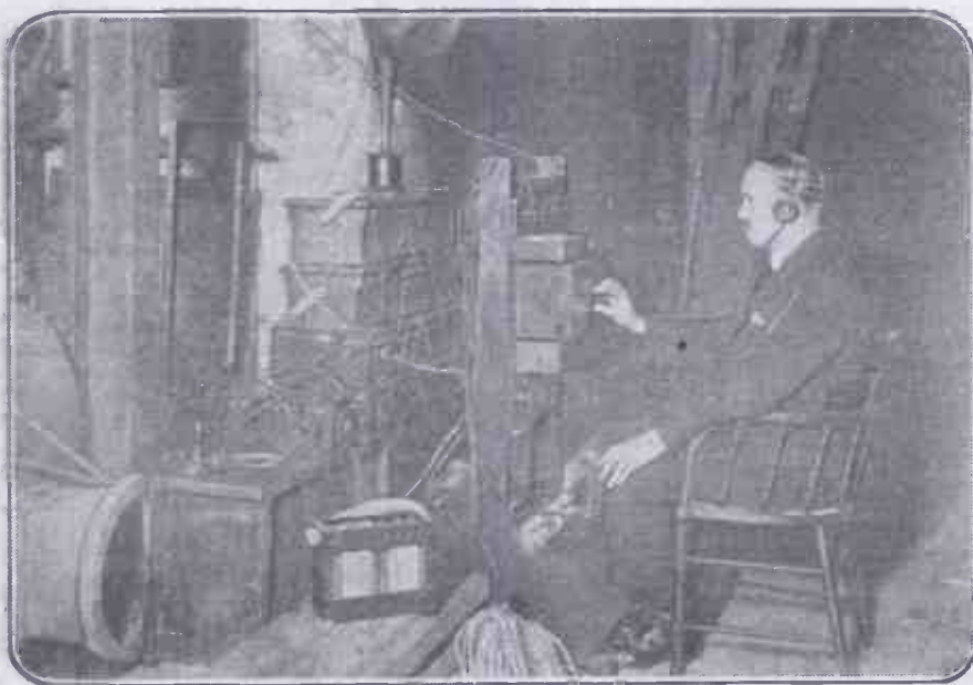
The amplifying apparatus under the stage at the Hippodrome. Land-line wires to 2 L O carry the strains of the familiar pantos.
