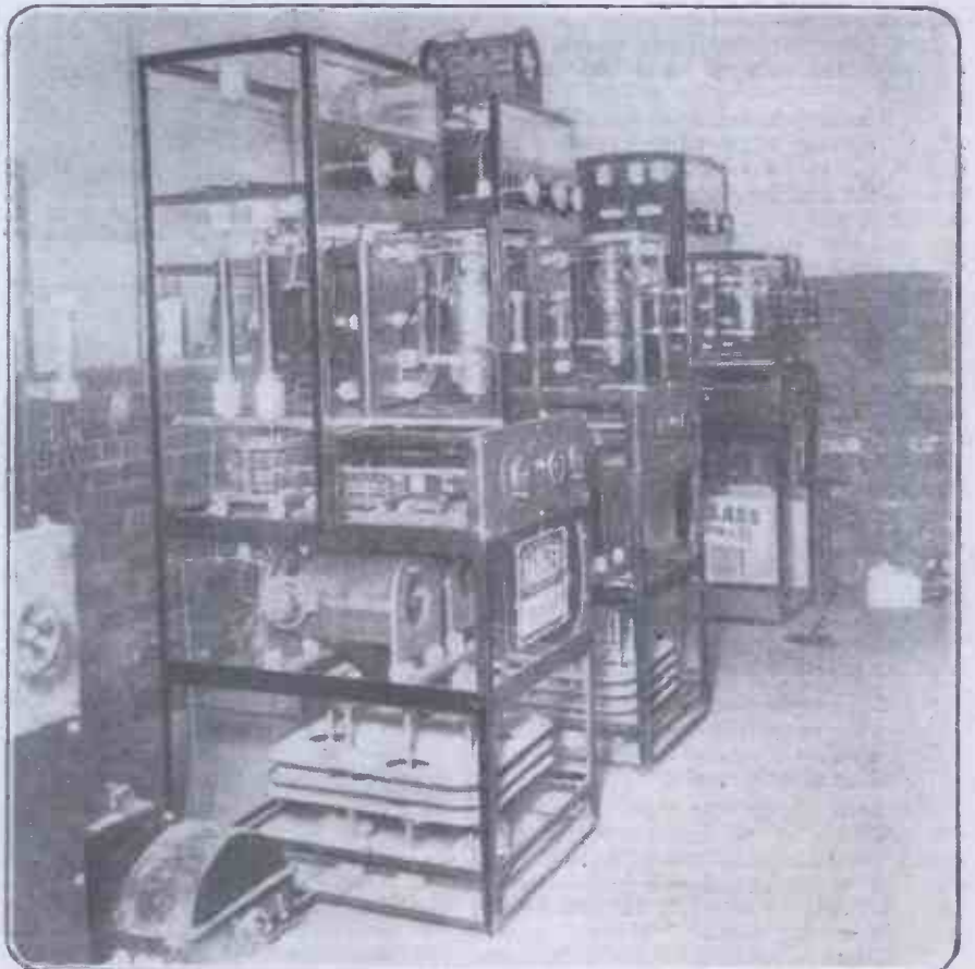
The valve-transmitting apparatus at the Cardiff Station of the British Broadcasting Co. These photos were specially taken for "Popular Wireless" by Mr. G. E. Thompson, of Cardiff.
