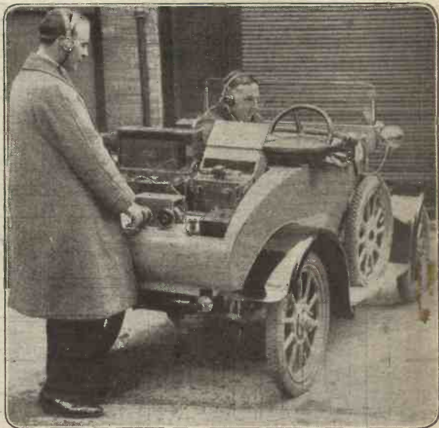
At a demonstration given by the Jowett Light Car Social Club the other day, a wireless set was fitted to a two-seater, and experiments were carried out. Good signals were received while the car was travelling at a fast speed.
