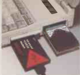
Two PCMCIA slots on all models provide ultimate expansion. Intel fax/data modem at an incredible £99 (except T3600)
