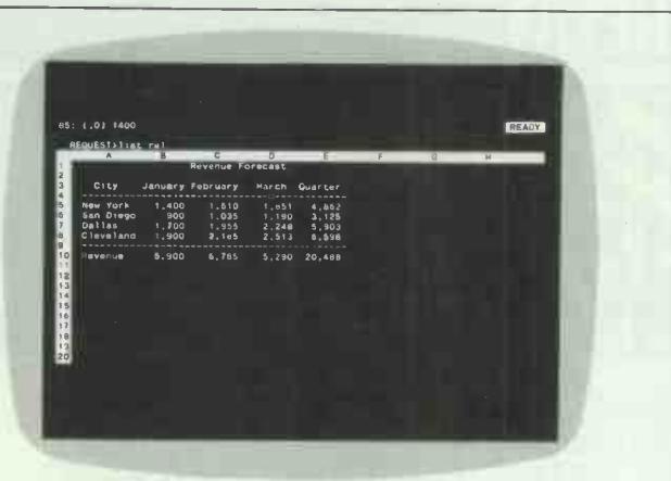
Finding where the formulae reside is all very well, but sometimes you need a way of quickly determining the relationships between various formulae. This is undertaken by the LIST REL command
