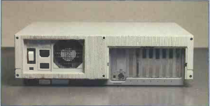
There are six 16-bit and two 8-bit slots on the back panel
