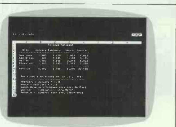
The LIST REL command is automatically placed directly below the current work, so that you can see both the relationships and the cells they refer to at the same time
