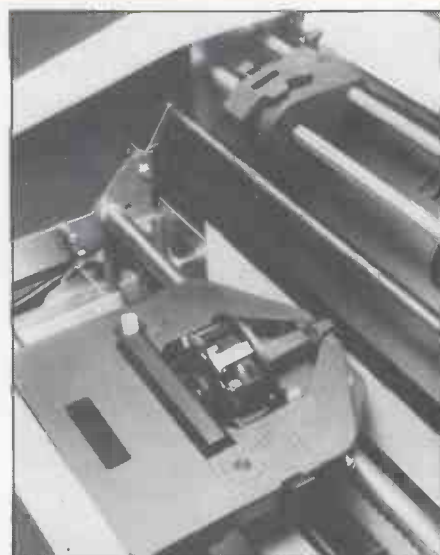
Print head and Facit ribbon cartridge
