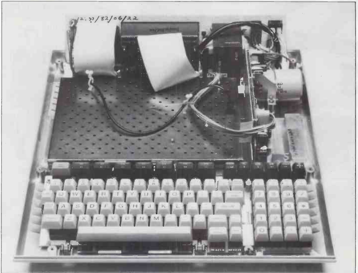
The perforated plate is a Faraday cage to trap RF emissions
