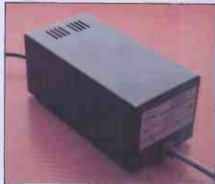
Power supply is 3-voltage
