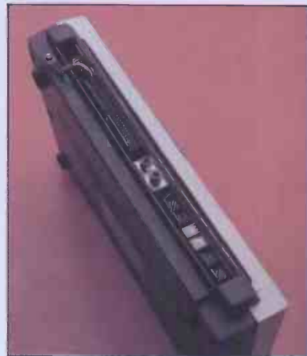
Socket panel is also a heat sink
