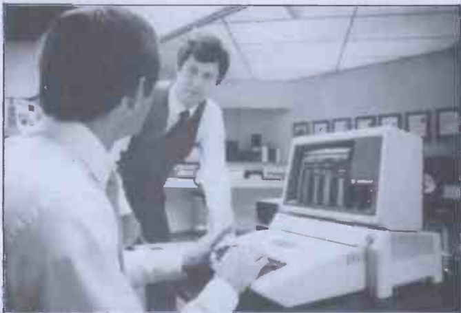
This may look like an attempt to disguise an Apple II as an Apple III — instead, it's a device which tries to tidy up the II by giving it a single on-off switch, a voltage surge suppressor, and fewer trailing cables, all for £125 (inc VAT). Details from Fletcher Dennys Systems, 01-570 8999.
