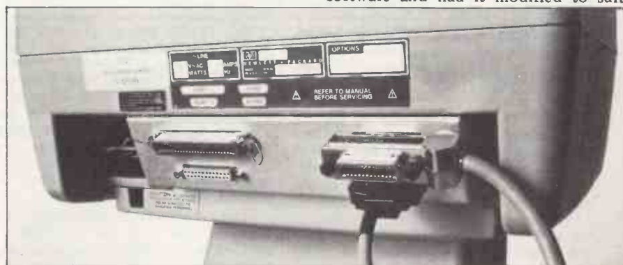
Note stacking connector for IEEE (HP-IB) port.
