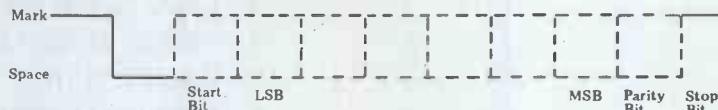
Fig 1 Serial data format. The duration of each bit is (1/baud rate) seconds.
