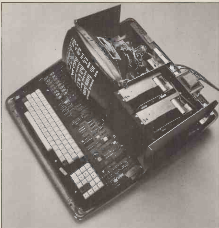
A trepanned SuperBrain — note the heavy shielding between CRT and disk drives.
