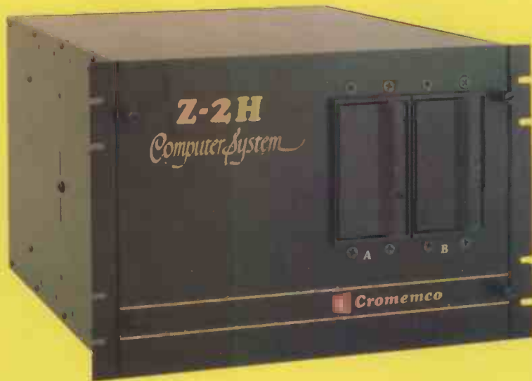
Cromemco Model Z-2H hard disc computer. 10 megabyte hard disc, 2 floppy discs, Z-80 computer and 64K memory. MicroCentre price £5,326.
