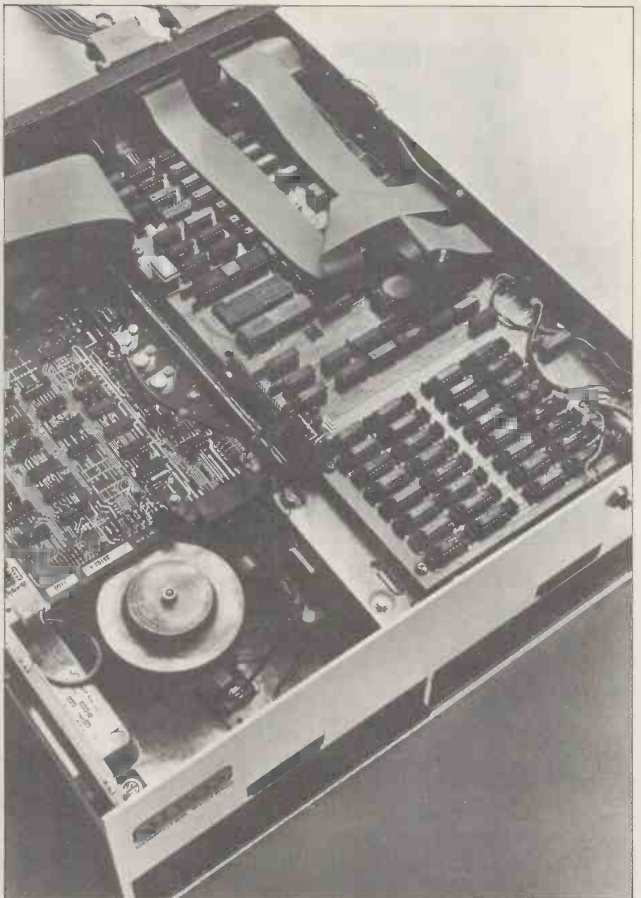
The processor/disc unit with its lid removed showing the single board computer to the right and one of the drives visible on the left.
