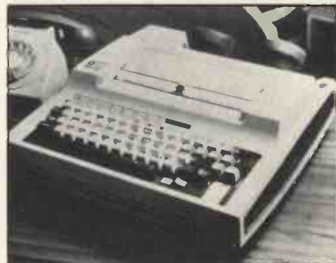
The Texas Instruments Model 765 portable bubble-memory data terminal, which retains data even when switched off.
