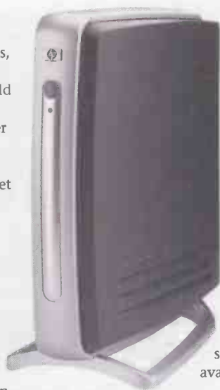
The HP Compaq t5500 is a mid-range thin-client device running Windows CE .Net and providing a local browser and legacy terminal emulation alongside the RDP and ICA clients
