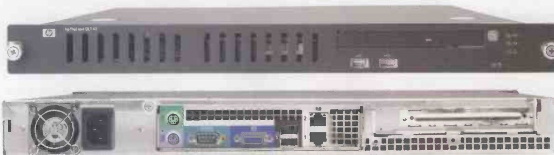
Top left (front view) and bottom left (rear view): The HP Proliant DL140 crams a lot of processing power into its slimline 1U case
