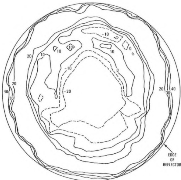
FIG. 9—Profile contour for Goonhilly 3: divergent wavefront
