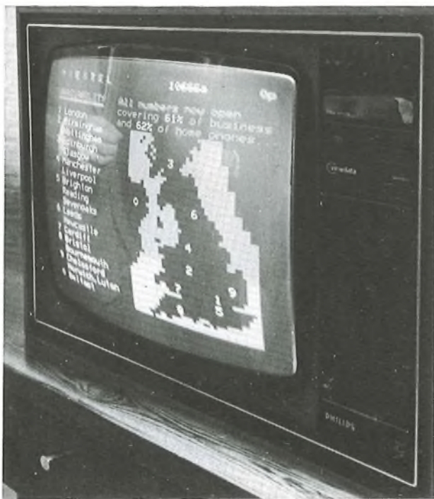
FIG. 1—Typical residential viewdata set, which uses a remote control tuner and keypad
