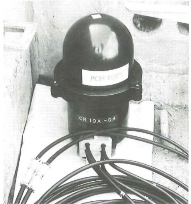
Note: the connectors in the tail cables are as used for export schemes and are not used by the BPO.
