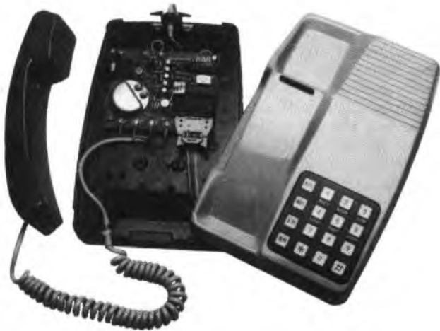
An experimental microprocessor telephone. (On this model, the sounds made by the tone-caller can be varied by pressing buttons on the keypad.)
