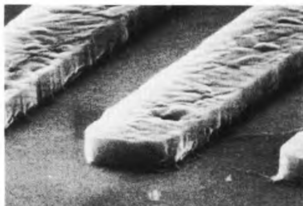
FIG. 10—Plasma-etched aluminium test structure (4 \mu m wide, 1 \mu m thick)
