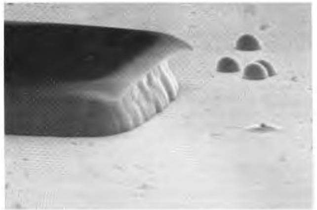
FIG. 13—Gold-plated individual heat sink, after replating, with photoresist still in place
