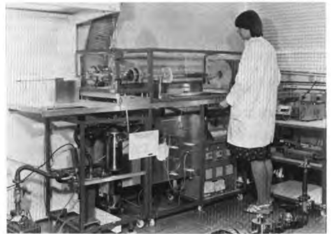
FIG. 3—Liquid-phase epitaxy kit
