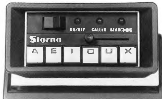
Fig. 4—Control box for the 55-channel mobile
