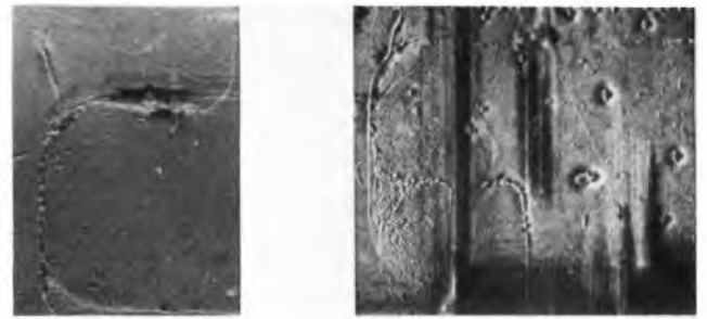
FIG. 10—X-ray Lang topographs showing layers of high and low crystallographic quality respectively on substrates of similar quality
