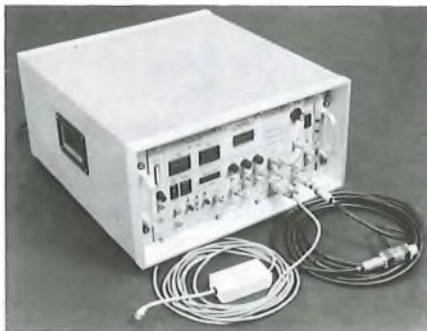
FIG. 6—The prototype through-pulse-echo cable tester
