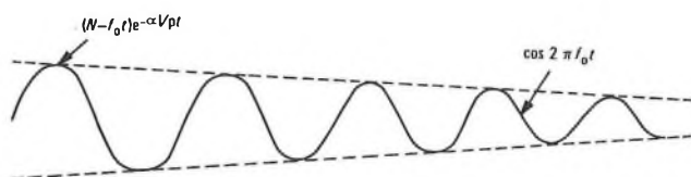
FIG. 3—The equalized forward-echo response of a coaxial cable with a single resonant structure
