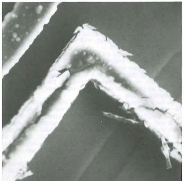
(b) Corrosion of single track
