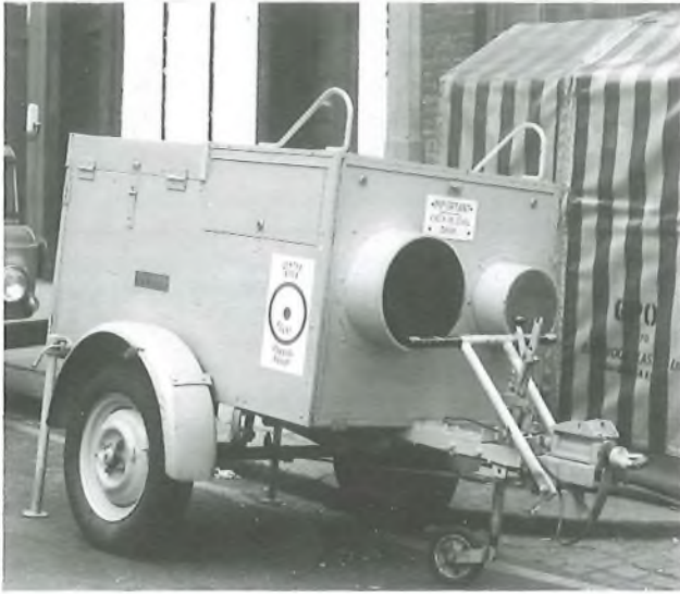
Self-contained trailer-mounted generator
