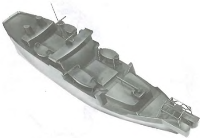
FIG. 2—The 1/60th scale model used for aerodynamic tests
