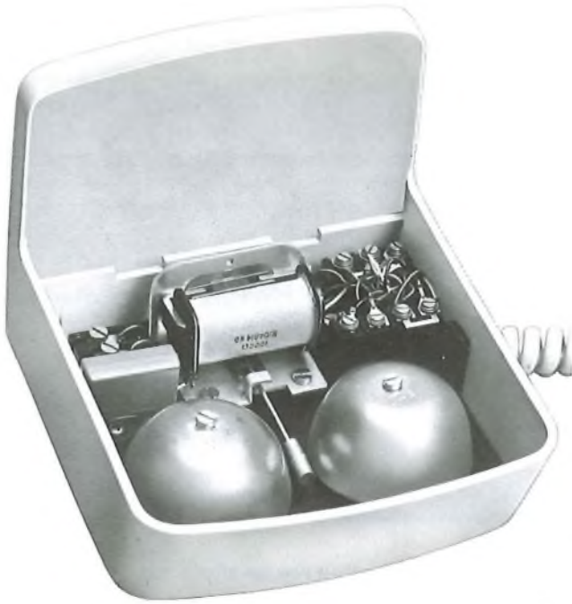
FIG. 4—Wall bracket with lid removed
