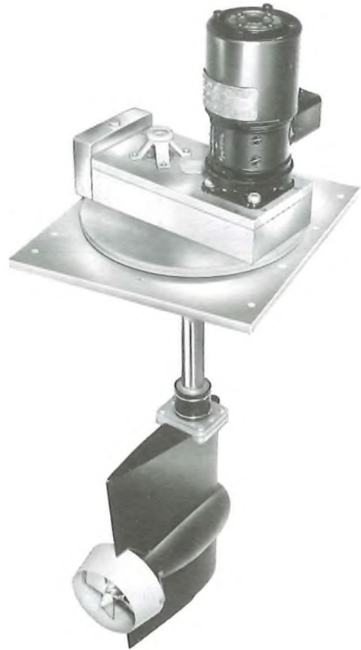
FIG. 6—Model of active-rudder unit
