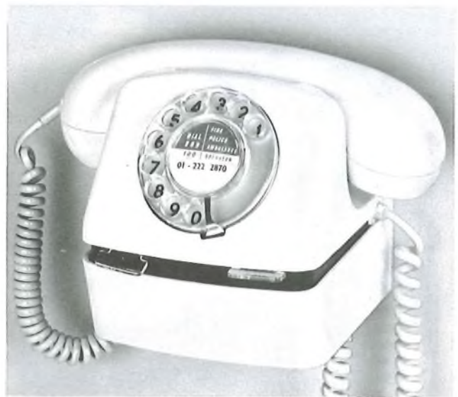
FIG. 2—New-style telephone with wall bracket
