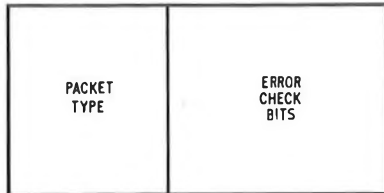
FIG. 5—Loop-delay-measurement packet structure
