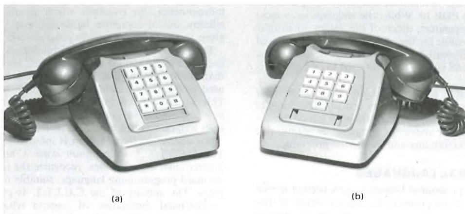
(a) Multi-frequency and d.c. code C signalling instrument (b) Loop-disconnect signalling instrument
