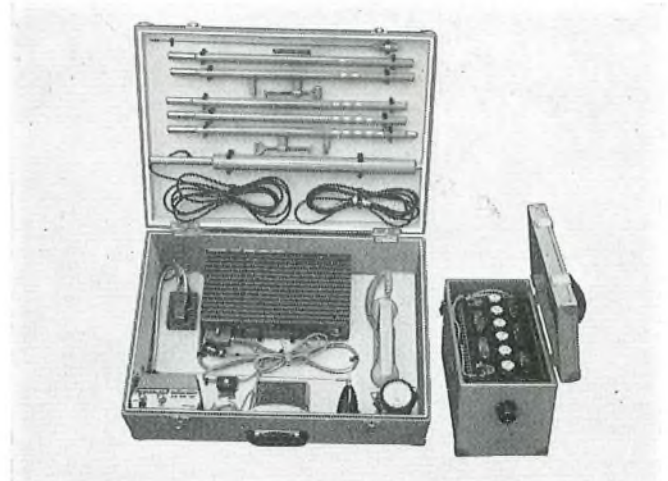
FIG. 1—An emergency radiophone unit complete with battery and aerials. The lid containing the aerials is removed before use.
