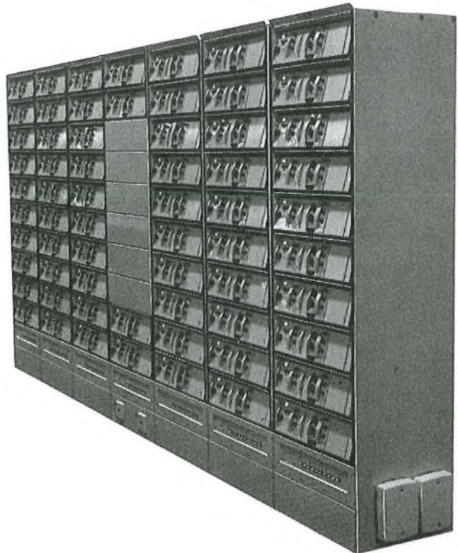
FIG. 2—Seven 62-type racks mounting Datel Modems 1D
