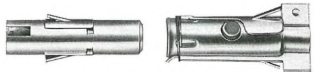
(b) Coaxial connector inserts
