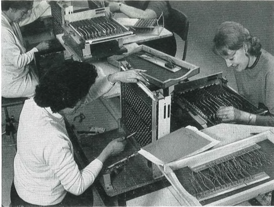
FIG. 4—Production of B-switches for TXE4 exchanges
