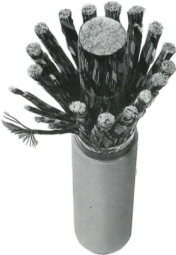
FIG. 3—A 4,800-pair cable with 0.32 mm copper conductors and solid-polythene insulation
