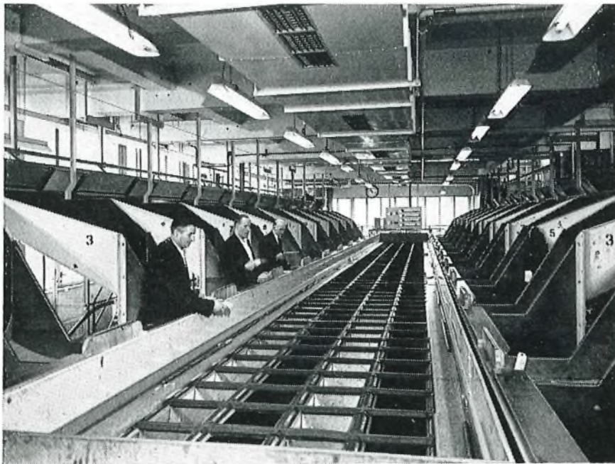
FIG. 11—Packet Sorting Machine at London Western District Office
