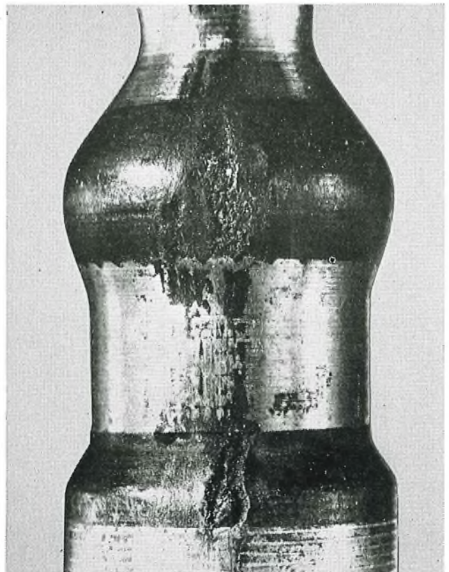
FIG. 9—Electrical tracking damage on unsuitable moulding material
