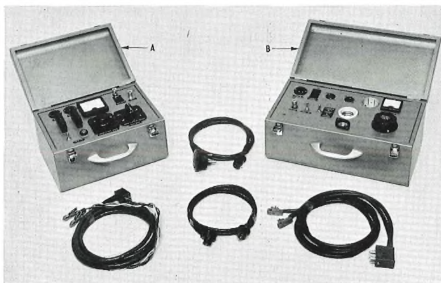
A—Emission tester B—Power-supply unit FIG. 1—EMISSION TESTER AND FILAMENT POWER-SUPPLY UNIT
