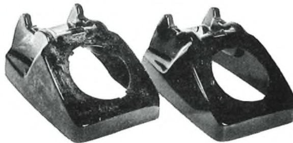
The right-hand case was wiped with Cetrimide solution, the left-hand case was untreated. Both were then polished and exposed to dust (cotton lint). THE EFFECT OF ANTI-STATIC TREATMENT OF TELEPHONE MOULDINGS
