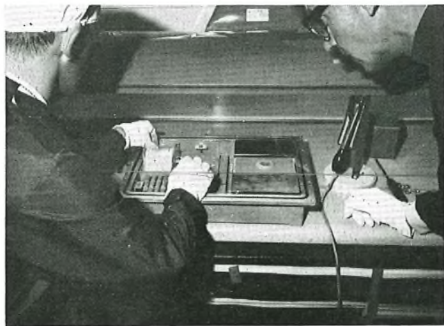
FIG. 6—SELECTING COMPONENTS ON THE SHIP FOR THE EQUALIZING NETWORK TO BE INSERTED IN A SUBMERGED EQUALIZER
