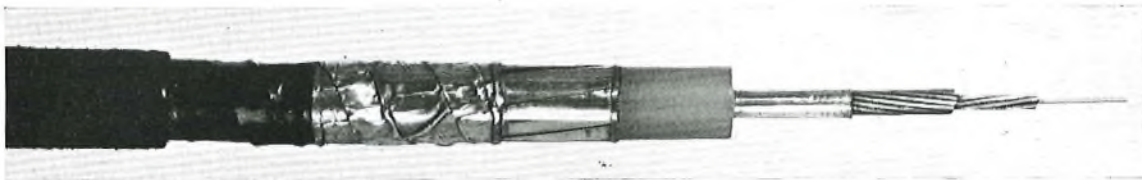
FIG. 2—FIRST EXPERIMENTAL LENGTH OF LIGHTWEIGHT CABLE
