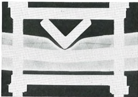
FIG. 6—RADIOGRAPH SHOWING DEFORMATION OF LIGHTWEIGHT CABLE BY A STEEL ANGLE AT A LOADING OF 0.75 TON
