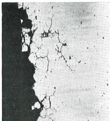
FIG. 1.—SURFACE PITTING AND CRACKS DUE TO INTERCRYSTALLINE CORROSION
